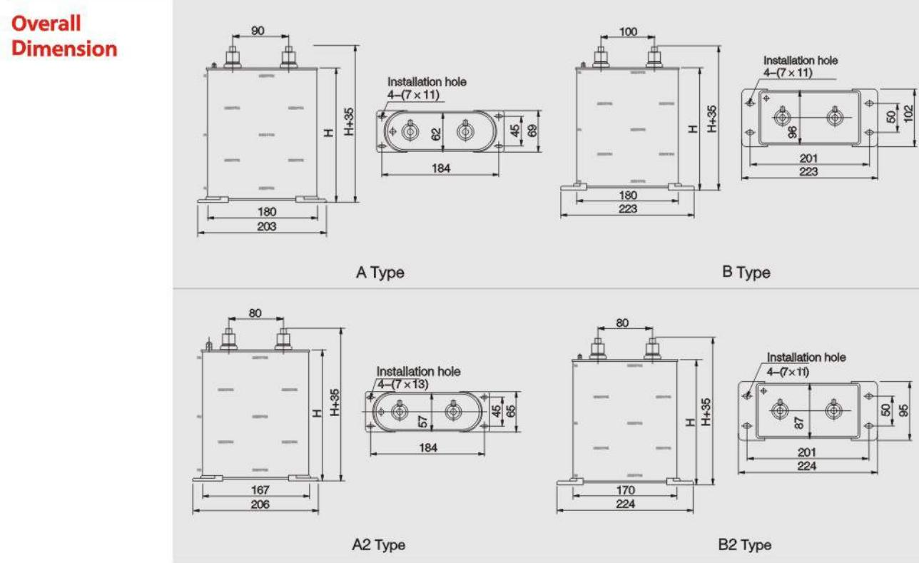
**Low voltage shunt capacitor
